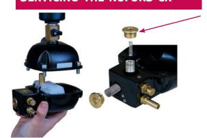
The NUFORS-CR design allows you to service the valve by unthreading one brass fitting. You have direct access to the valve plunger and orifice.
